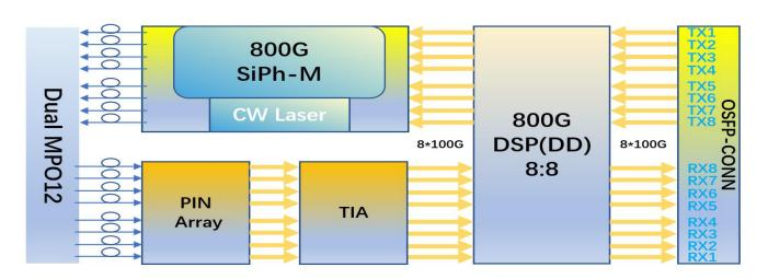
Figure 1. DR8 Module Block Diagram
