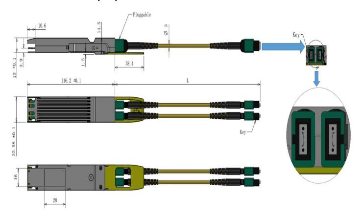
Figure 10. Mechanical Specifications
