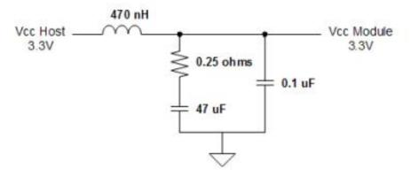
Figure 8. Host Board Power Supply Filtering
