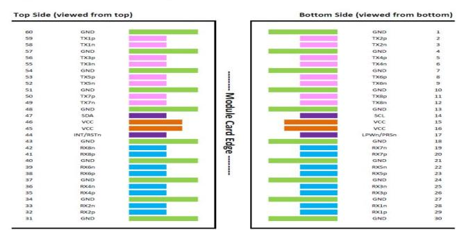
Figure 3. OSFP module Pin-out Details
