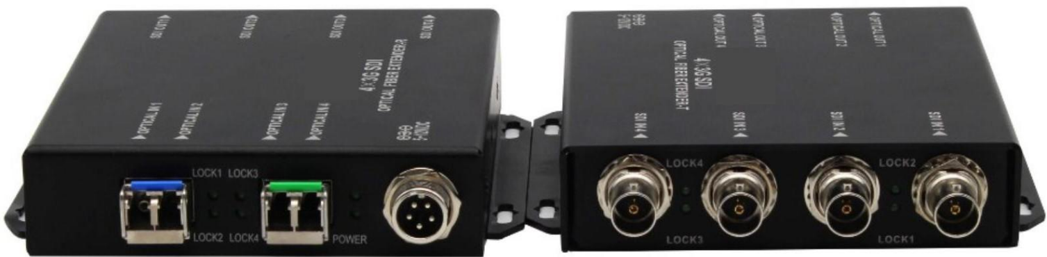
Figure3. Mechanical Specifications of 4x3G SDI Extender: (a) 4x3G Transmitters; (b) 4x3G Receivers
