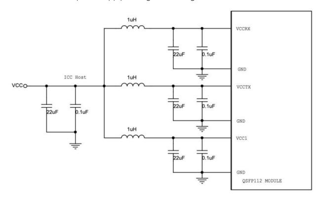
Figure 3. Host Board Power Supply Filtering
