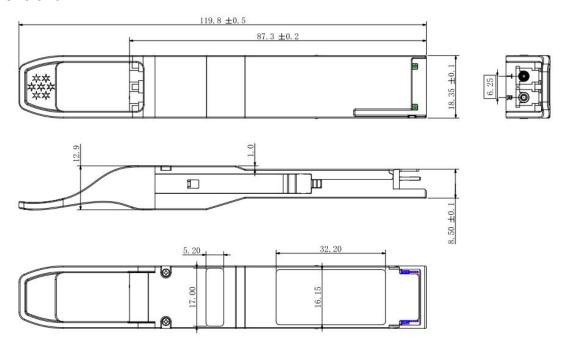
Figure 5. Mechanical Specifications
