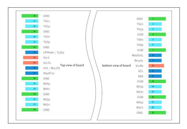
Figure 2. QSFP112 Module contact assignment
