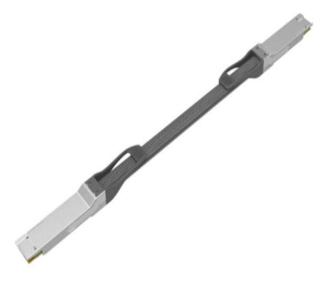
FIBERSTAMP's FZJ-400xxxxC cable connects data signals from each of the 16 pairs on the single QSFP-DD end to the other QSFP-DD end, each pair operates at data rates of up to 50Gb/s and can be adaptive downward compatibility. The product operates 3.3V power supply and comply with QSFP-DD-MSA and IEEE802.3cd ,it's high performance & cost effective I/O solutions for LAN, HPC and SAN. The high speed cable assemblies meet 400Gigabit Ethernet, Infiniband requirements for performance and reliability.
