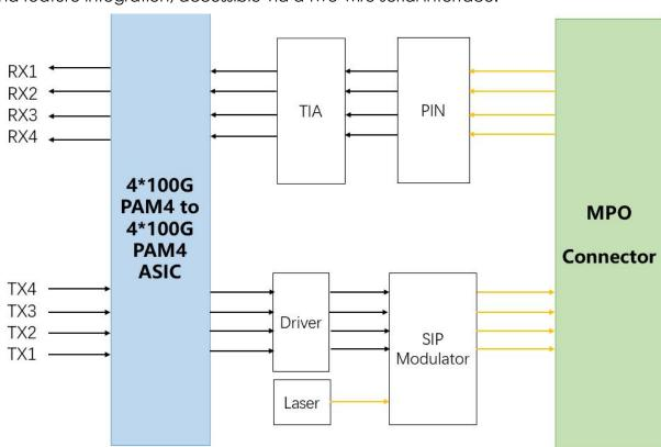
Figure 1. Module Block Diagram
