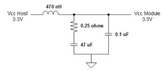
Figure 3. Host Board Power Supply Filtering
