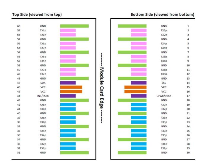
Figure 2. Electrical Pin-out Details
