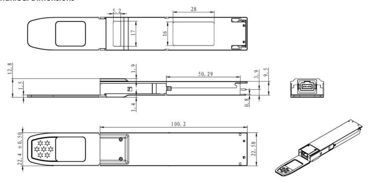
Figure 5. Mechanical Specifications
