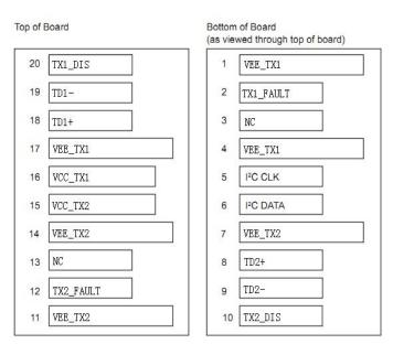
The I2C bus interface uses the 2-wire serial CMOS E2PROM protocol. The serial interface meets the following specifications:
