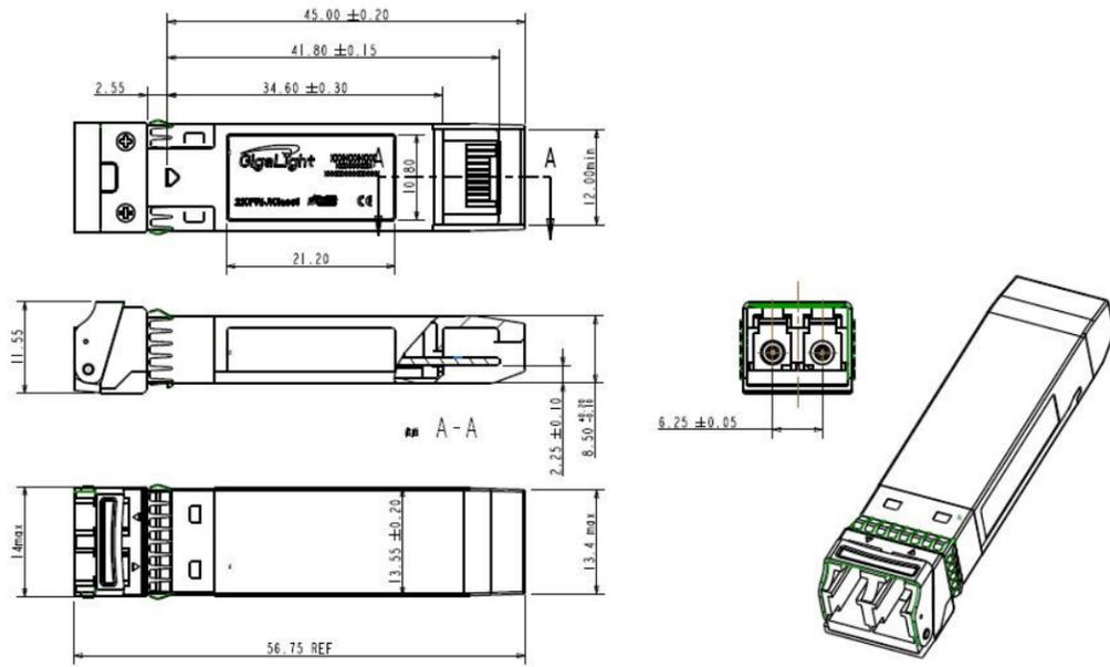
Figure4. Mechanical Specifications
