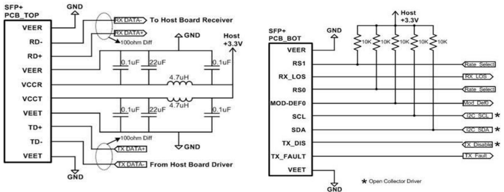
Figure3. Recommended Interface Circuit
