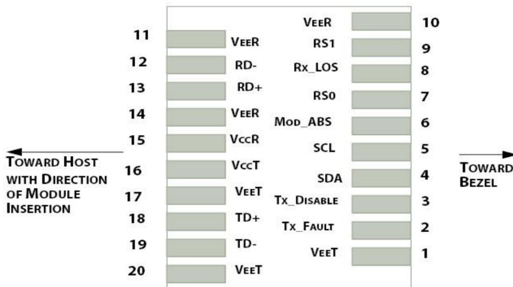
Figure2.Electrical Pin-out Details
