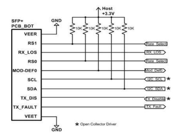
Figure3.Recommended Interface Circuit
