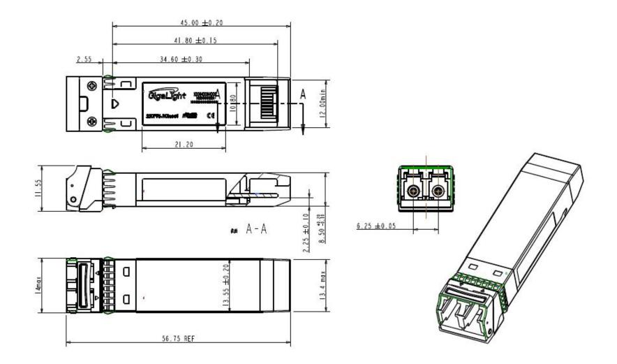
Figure 4. Mechanical Specifications
