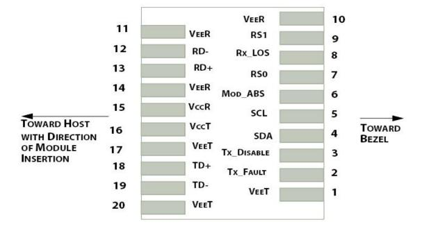
Figure 2. Electrical Pin-out Details
