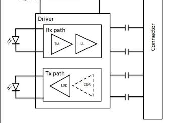
Figure 1. Module Block Diagram
