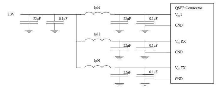
Figure 4. Host Board Power Supply Filtering
