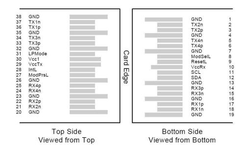
Figure 3. Electrical Pin-out Details
