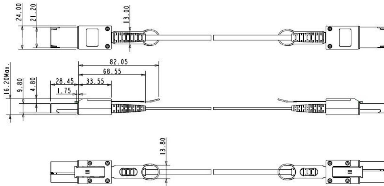
Figure6. Mechanical Specifications
