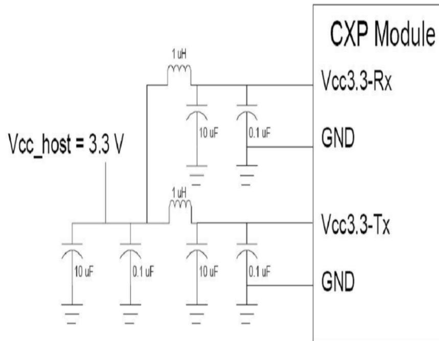
Figure3. Host Board Power Supply Filtering
