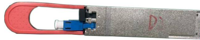
FBG-112L4K40CL transceiver with attenuator (for reference
