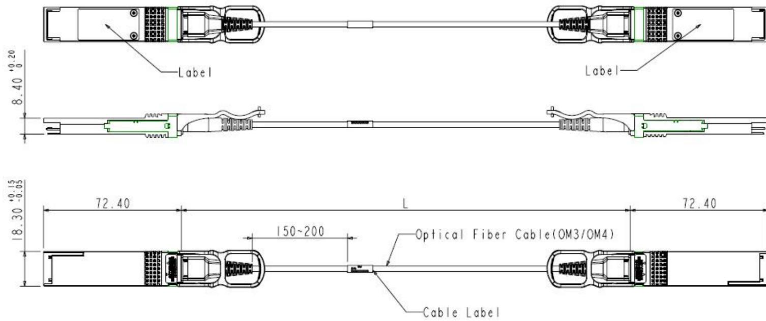
**Figure 9. Mechanical Specifications**
