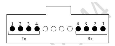
Figure 4. Optical Receptacle and Channel Orientation
