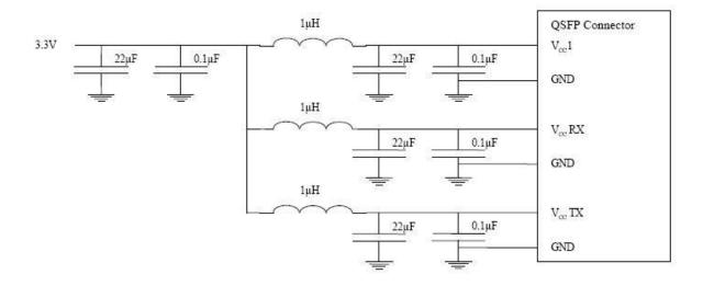
Figure 3. Host Board Power Supply Filtering
