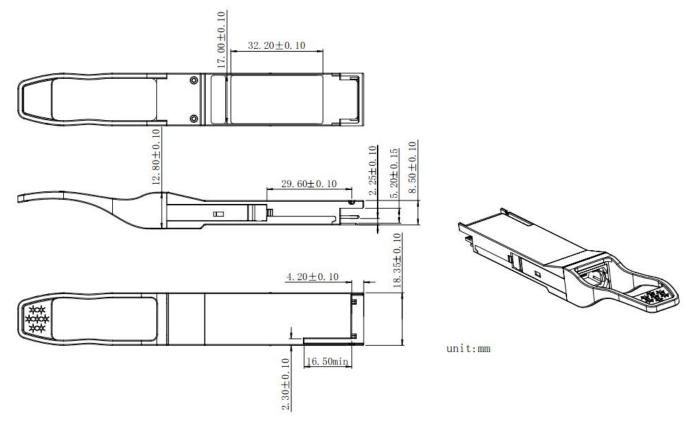
Figure 9. Mechanical Specifications
