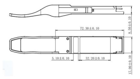
Figure 8. Mechanical Specifications
