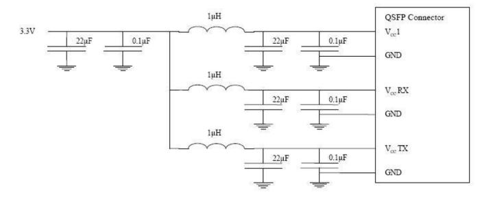
Figure 3. Host Board Power Supply Filtering
