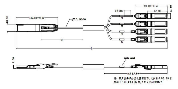
Figure 1. Mechanical Specifications
