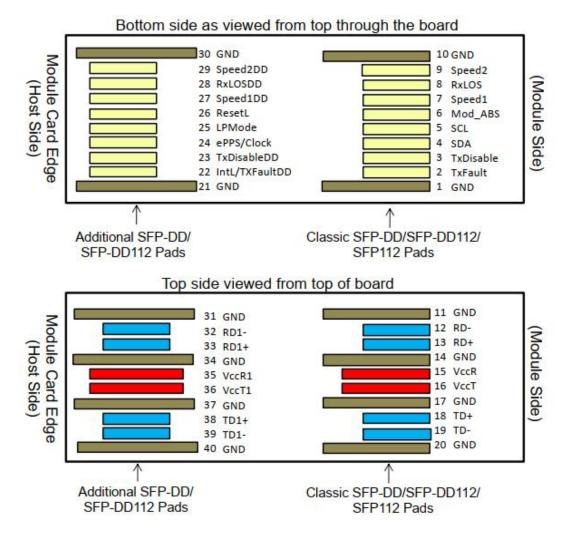
Figure 2. Electrical Pin-out Details
