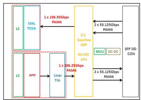
Figure 1. Module Block Diagram
