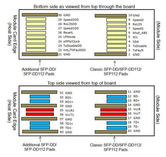
Figure 2. Electrical Pin-out Details
