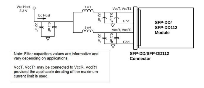
Figure 3. Host Board Power Supply Filtering
