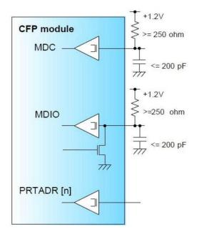
Figure 5: Reference MDIO Interface Termination
