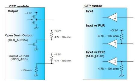
Figure 3: Reference 3.3 V LVCMOS Input / Output Termination
