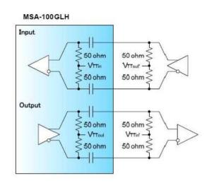
Figure 2: High-Speed I/O for Data and Clocks
