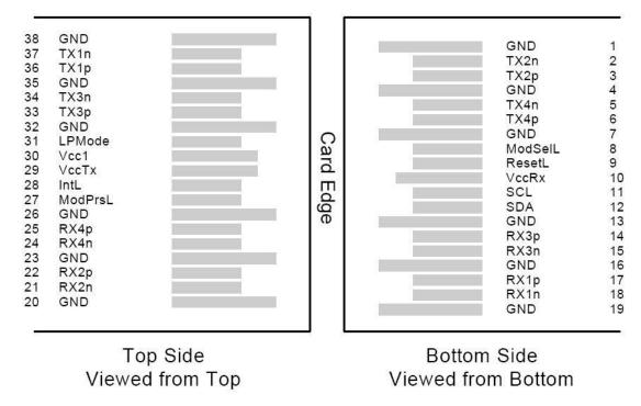
Figure 2. Electrical Pin-out Details
