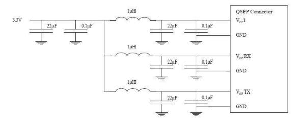
Figure 3. Host Board Power Supply Filtering
