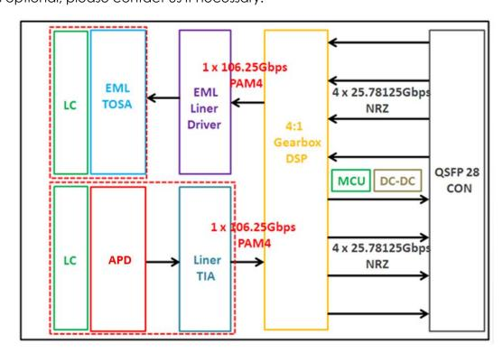
Figure 1. Module Block Diagram
