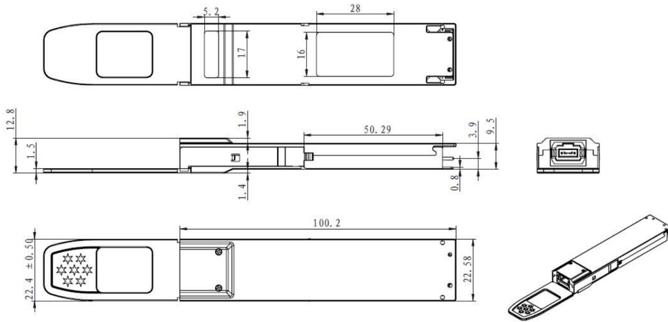
**Figure5. Mechanical Specifications**
